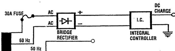
Normal AC voltage running to the rectifier (while the engine is operating at 3600 rpm) is measured across the two AC connections on the bridge rectifier.
