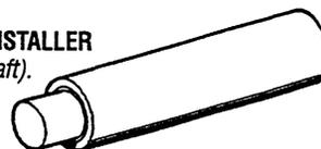
**PIN** *For supporting the sprocket when the camshaft sprocket is loosened or tightened.*
