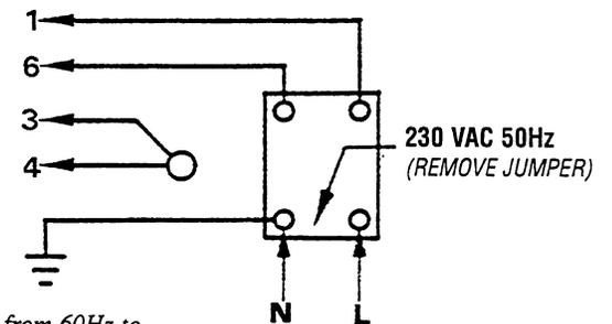
**NOTE:** When changing from 60Hz to 50Hz, make certain the ground wire is properly repositioned according to this diagram.
