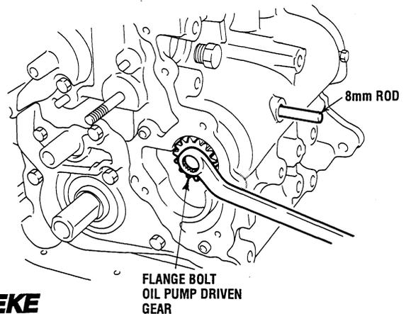
2. Remove the oil pump cover and gasket. Discard the gasket.
