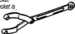
**CRANKSHAFT FRONT OIL SEAL INSTALLER**
