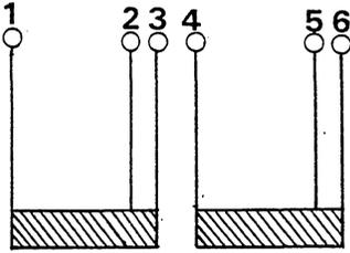
**Group #1** - Measure resistance value between terminal with lead #1 and terminal with lead #3. (Check that there is no continuity of Group #1 windings to the case ground).
