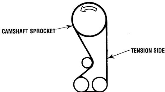
7. Loosen the temporarily tightened tensioner nut on the water pump side 1 or 2 turns, and tension the belt making use of the spring force.
