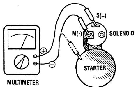
**NOTE:** Disconnect the wire from terminal M.
