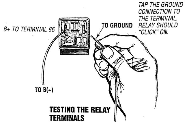
TESTING THE RELAY TERMINALS
