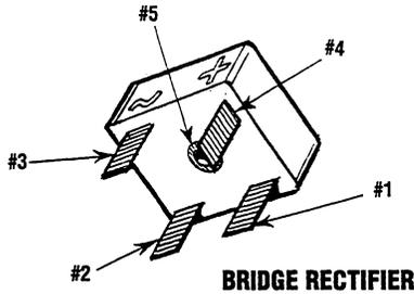
4. Leaving the negative multimeter (-) lead on point #4, touch point #5 with the positive lead. No deflection should take place.
