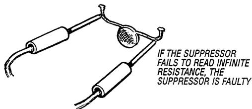
IF THE SUPPRESSOR FAILS TO READ INFINITE RESISTANCE, THE SUPPRESSOR IS FAULTY
