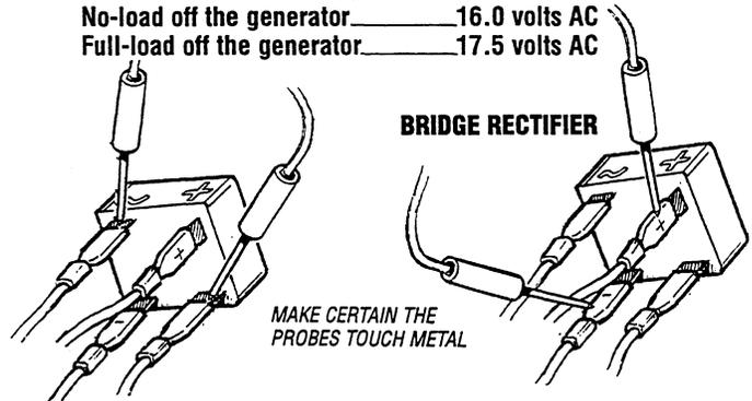
Normal DC voltage running out of the rectifier (in volts DC) is measured across the two DC connections of the bridge rectifier, that is + and -.
