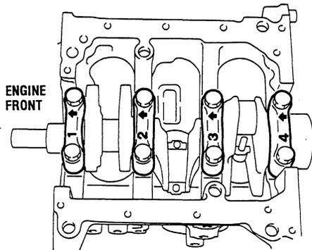
2. Install the bearing cap paying careful attention to the cap number and the arrow mark. Apply oil to the bolt threads.
