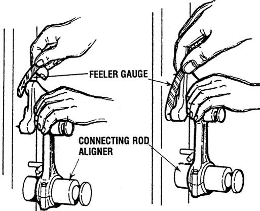
CONNECTING ROD TWIST LIMIT 0.004in (0.1mm)
