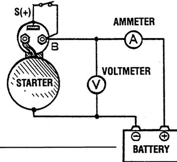
**CAUTION:** Use thick wires as much as possible and tighten every terminal securely. This is a solenoid shift-type starter which makes a rotating sound louder than that of a direct-drive type starter. When detecting starter rotation at the pinion tip, be careful not to come in contact with the pinion gear when it protrudes.
