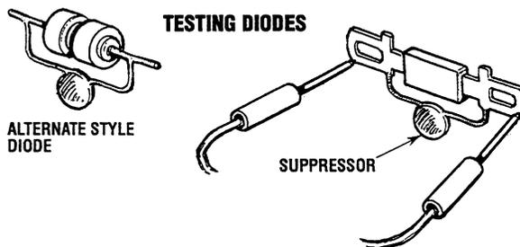
Both diodes should measure the same resistance value. If one measures lower than the other, it is presumed faulty. Replace both.
