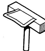
**CRANKSHAFT REAR OIL SEAL INSTALLER**
